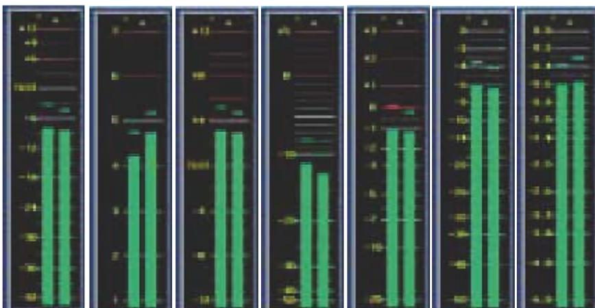
Type I Nordic Type IIa BBC Type IIb EBU DIN VU Digital Digital zoom
