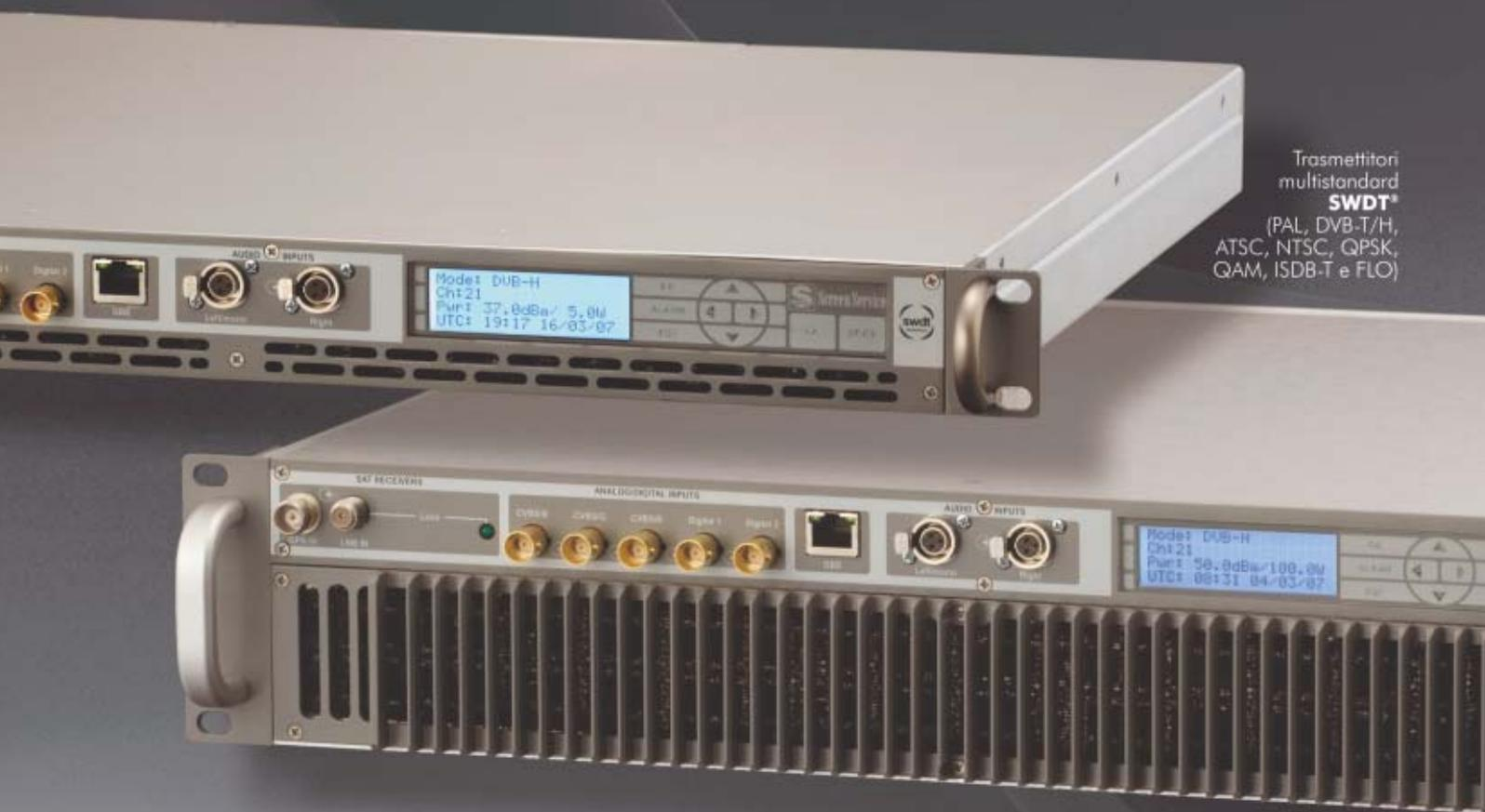
Trasmettitori multistandard **SWDT\*** (PAL, DVB-T/H, ATSC, NTSC, QPSK, QAM, ISDB-T e FLO)
